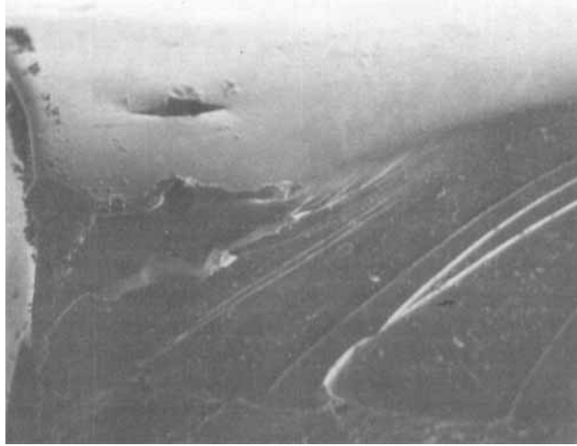
FIGURE 7 SEM photograph of the bending fracture surface.
