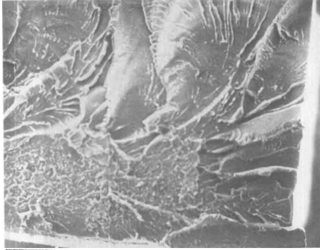
FIGURE 9 SEM photograph of notched edge at higher magnification.
